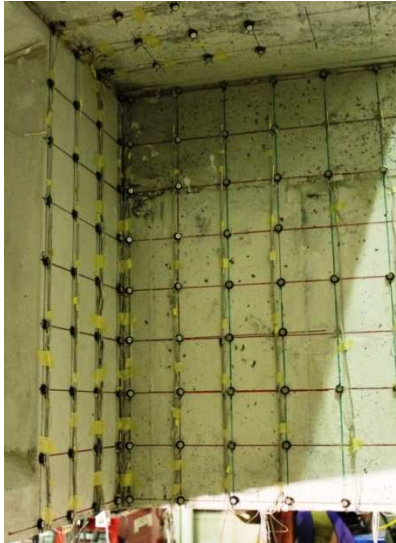
Figure 4.12. LED indicators to record position during experimental testing
